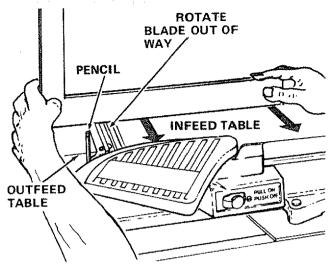
It is easier to adjust the infeed table while the Jointeris setting on your workbench.
